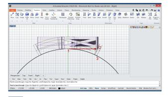
Now, still in the right view, under the Transform Tab with the Bend tool to adjust the solid to the pretended curve. It's important to act vate the symmetry option in the command line.
