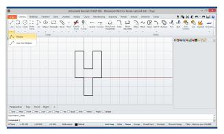
Under the Drawing tab, with the Polyline tool, we can define the pretended shape and dimensions in the top view, as the above image.
